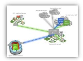
The Athens platform will be implemented on the Athens.5Glink (www.athens5glink.eu) testbed. The testbed is going to be extended to offer the telecommunication ecosystem an E2E experimental 5G platform, showcasing features of next generation networks, with particular focus on software network technologies (NFV/SDN) and edge computing for small cell infrastructures.
